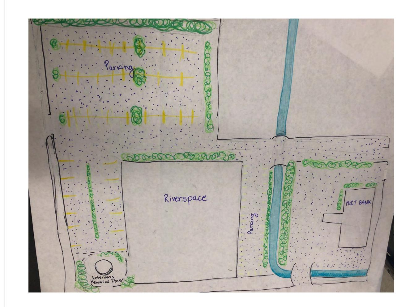
Note the new daylighted river and vegetation, as well as the permeable pavement to reduce flooding and increase this area's appeal.
